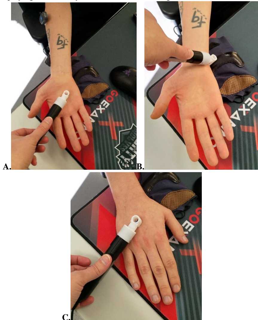
Figure 1.6. Wrist skin moisture testing process with Tewameter (A. on the volar (palmar) surface of the wrist; B. on the wrist basement; C. on the dorsal surface of the wrist)
